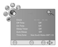
When the Auto Sleep is set to ON, the unit will turn to standby mode automatically if there is no signal input for a period of about 15 minutes.
